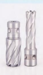
四孔柄系列 柄径Φ18.0mm, 特征在于90度分布4点定位孔。 适合用于 FEIN 系列磁座钻机。 HSS annular cutter with FEIN Quick-in Shank, the diameter of shank is Φ18.0mm, which is suitable for 90° distribution at 4 locating holes. FEIN Quick-in Shank, suitable for FEIN magnetic drills.
